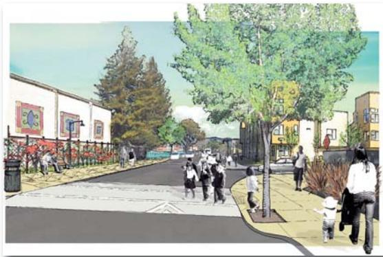
**Figure 1.** A complete street concept adjacent to an inner-city low-income housing project includes raised table crosswalks, bulb-outs to reduce crossing distance and provide room for trees, and decorative murals and vines on trellises within the narrow right of way.
