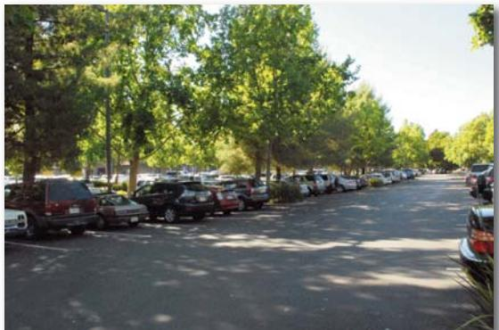
**Figure 6.** Ample tree canopy in a Danville Costco parking lot significantly reduces heat reflected from asphalt paving and cools ambient temperature by more than 15 degrees. Photo: Sarah Sutton
