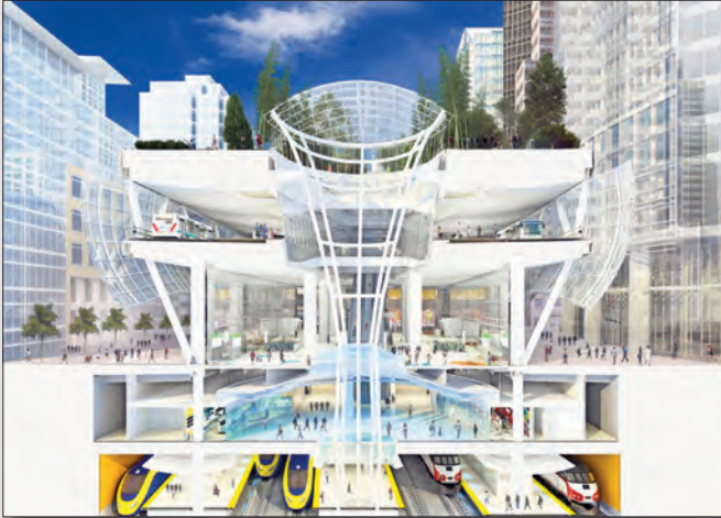
Figure 2. Cross-section of terminal. Top to bottom: 5.4-acre park; bus terminal; street-level entry concourse; lobby, ticketing, and gates for HSR and Caltrain; and train platforms. Source: TransbayTerminal.org media-gallery. http://bit.ly/jzSLwp
