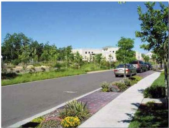
**Figure 5.** Proposed redesign alternates permeable paving strips for vehicle access with low-growing, colorful, drought-tolerant plants. Photo simulation: The Planning Center | DC&E
